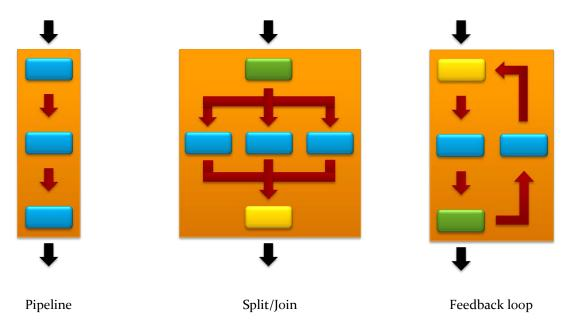
The atomic elements of a StreamIt graph are filters. All computation takes place within these filters, and each filter has a single input stream and a single output stream. Note that each of the composite graph constructors also has this property. Many of the graph operations performed by the StreamIt compiler rely on the structured nature of the graphs to simplify the analysis.
